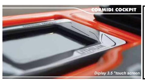
Diplay 3.5 "touch screen allows you to view all the settings of the machine as well as choosing the level of power and speed of the machine.
