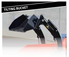
The tilting bucket not only load the dumper but can unload it frontally
