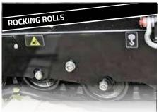
The machine's undercarriage oscillated to follow the terrain profile for increased stability and comfort and lifetime of crawler
